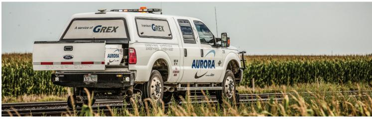
The lowa Interstate Railroad used the GREX Aurora® tie inspection system to evaluate the tie condition of more than 120 miles of track.
